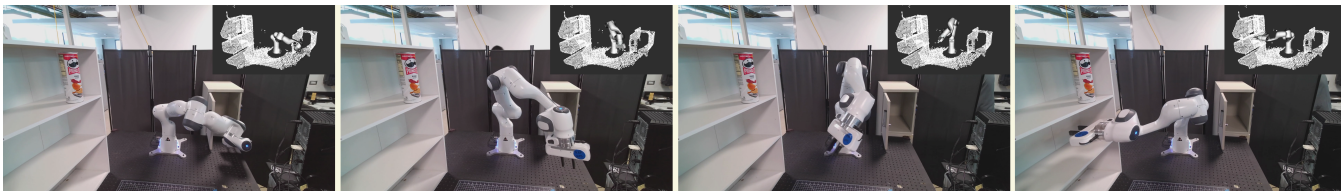
Fig. 6. Snapshots of a trajectory planned using VQ-MPT on a physical Panda robot. VQ-MPT generalizes to real-world sensor data without any additional data collection or fine-tuning and reduces planning time for finding near-optimal paths.
